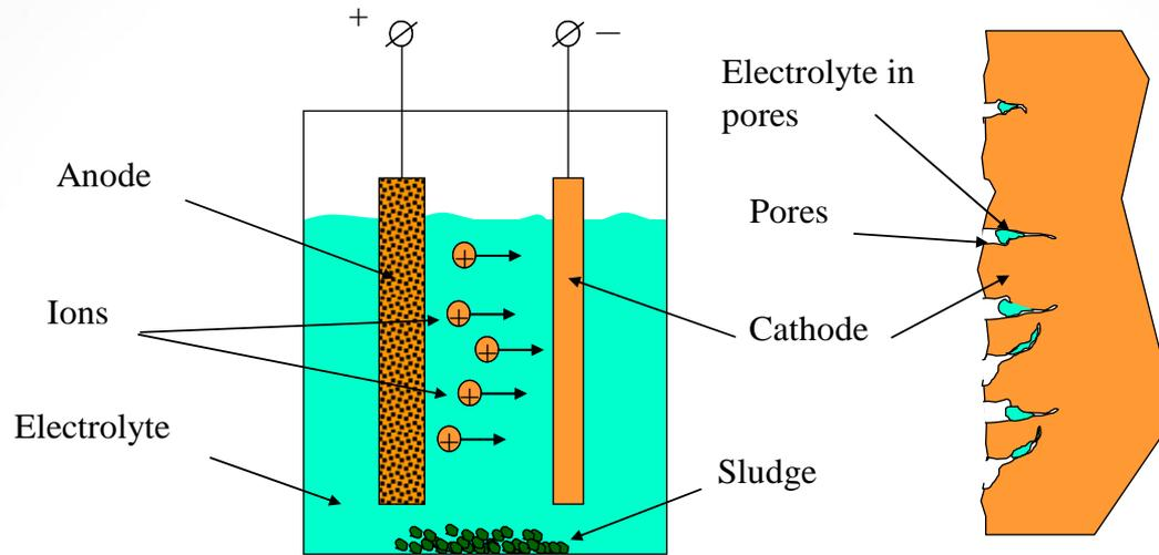
In an electric refining process, electrolyte enters the small pores that have developed on the surface of the copper sheets.
